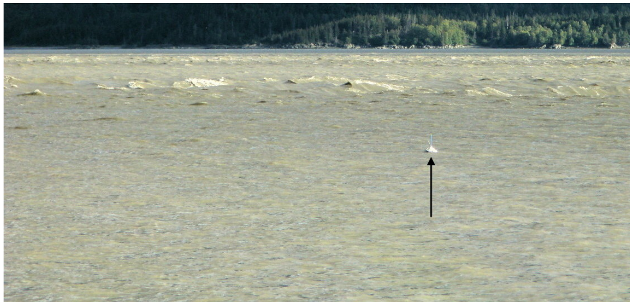
Figure 5. Recording platform deployed during ebb tide. The arrow indicates the remote-controlled boat. The boat approached turbulent waters but did not enter them, allowing measurement of propagating sounds with minimum exposure to near-surface turbulence that could introduce mechanical noise artifacts.
