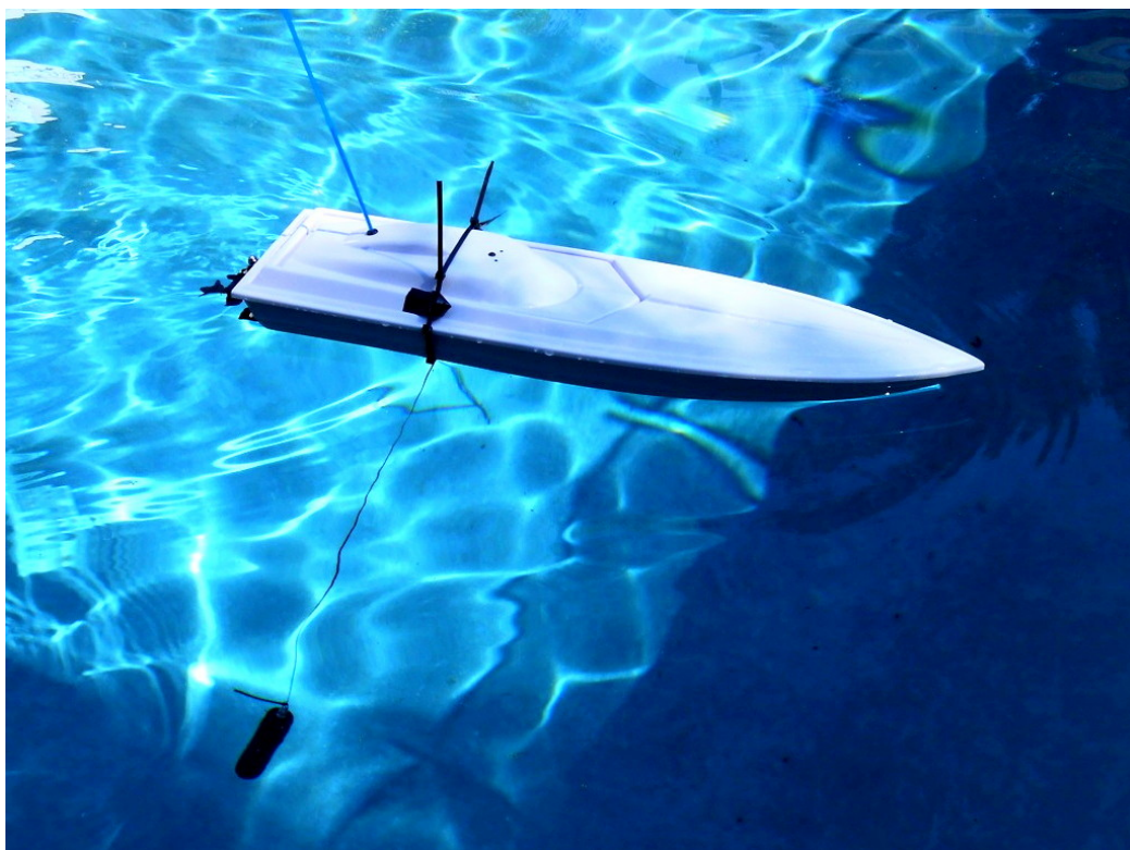
Figure 4. Recording platform. The remote-controlled boat is shown towing an Acousonde™ acoustic recorder at 39-in (1-m) depth during pool tests. The photograph does not show the retrieval-line fairing system, “beaver tail” foul guard, and eyebolt tie-off point that were added before deployment.
